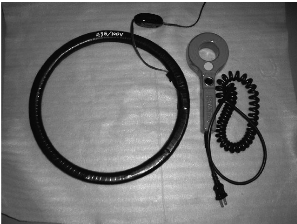
Fig. 8.3 De-magnetizers; 28cm internal radius coil (left) and handy coil (right).
